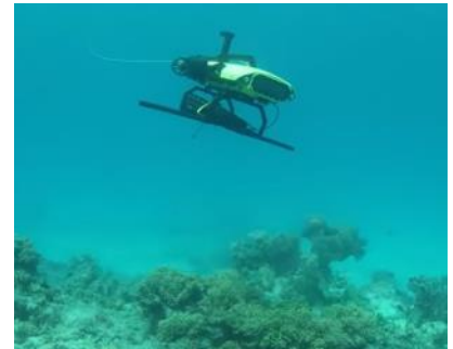
The LarvalBot in action, dispersing thousands of coral larvae. Photo: Queensland University of Technology.
