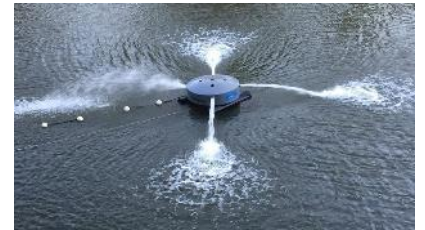
Aerators, such as this one, are being used to get more oxygen into the water. Photo: OzFish Unlimited.
