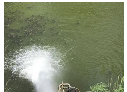
Some irrigators have reversed their pumps, creating localised areas with more dissolved oxygen and many fish are taking advantage. Photo: Sourced from https://bdtruth.com.au/main/news/article/10476-Reverse-pumping-working.html .
