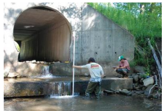
Assessments of culverts across the Hudson River catchments is helping local authorities improve local road infrastructure while at the same time reducing stream habitat fragmentation. Photo: https://www.tu.org/blog-posts/tu-works-in-new-york-to-improve-habitat-boost-flood-resiliency .
