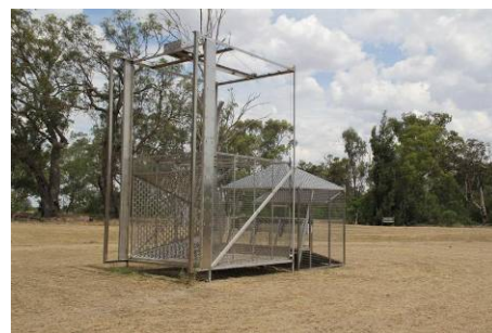
A carp separation cage waiting for high enough water flows to allow installation in the Macquarie Marshes. Photo: Sam Davis.
