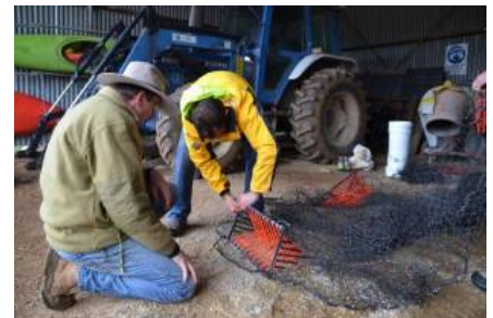
The carp trap being used in this trial is fitted with 'push entrances' which discourage native fish from entering the trap. Image source: bushheritage.org.au
