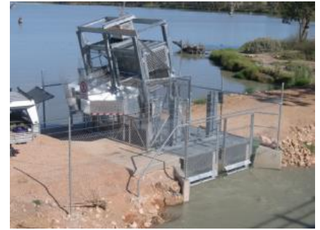
A carp trapping cage uses natural behaviour to trap the carp. Photo: Finterest.
